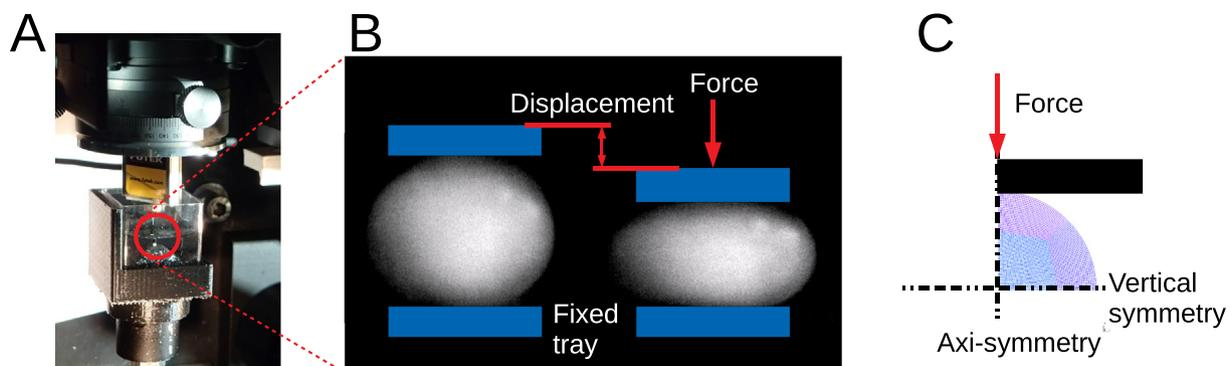
**Fig. 1.** Global compression test on micropellets. (A) Image of the device used for the mechanical characterization. (B) Schematic representation of the compression test (exaggerated deformation). (C) Symmetry assumptions used with the Finite Element model to estimate the micropellet hyperelastic properties.
